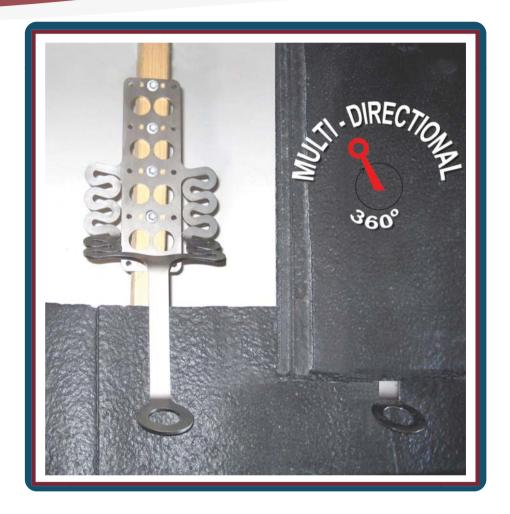
Its sleek design means fixing to a rafter is a simple task of screwing five (12 gauge, 50mm roofing screws) through the TileLinks existing holes. Five alternate fixing rows enable the TileLink $^{\text{TM}}$  to be positioned to suit the pattern of the roof tile. The TileLink fits snuggly between the existing tile eliminating waterproofing issues.
